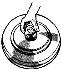
1 Removing Arming Plug From Mine.
