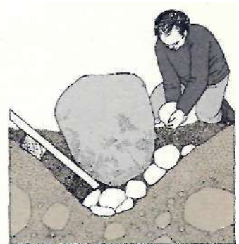
Raise the boulder as far as possible. Prop up with stones. Take lever and fulcrum to the other side.
