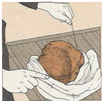
Use a wire to cut a workable lump from your store of pug.
