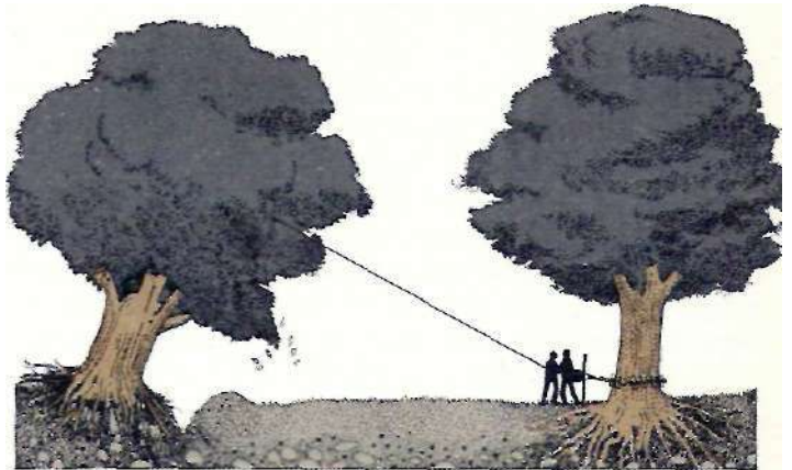
Using a monkey-winch Use the base of one tree as a hold-fast and attach the wire rope as high as you can to the tree you
