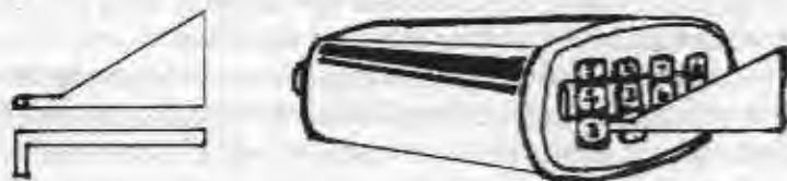
Figure 28. Manipulating the sesame padlock.
