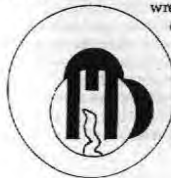
Figure 16. Protective inserts on the face of high-security cylinders.
