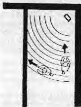
Figure 94. The ultrasonic motion detector is also most sensitive to movement directly toward or away from the sensor.
