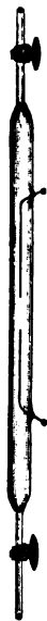
FIG. 97. On exposing one of these bulbs to the light of burning magnesium the combination of the two gases instantly takes place, with a sharp explosion which shatters the bulb to powder. The bulb should therefore be screened, as shown in Fig. 96.
