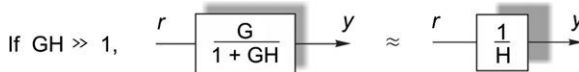
Figure A1.5 Simplification of closed-loop system model when loop gain ( GH ) is much greater than 1.
