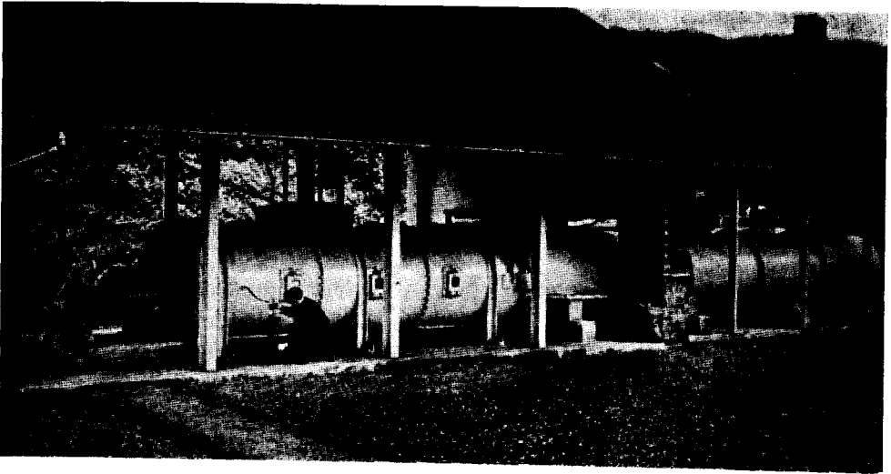
FIG. 154. Experimental gallery at I.C.I.'s Ardeer factory, according to J. Taylor and Gay [4] (a replica of Home Office Testing Gallery).
