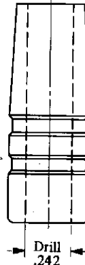
PIN, TUBULAR DOWEL (LARGE) FXS 535 - Type 1 Steel-WDX1112 (S.R.Q. Macro Etch) Class A Powdered Iron - Class B - Hardened Steel Tubing - Class C Finish Wt 197 Grs Approx For Other Dimensions See Drawing A299569
