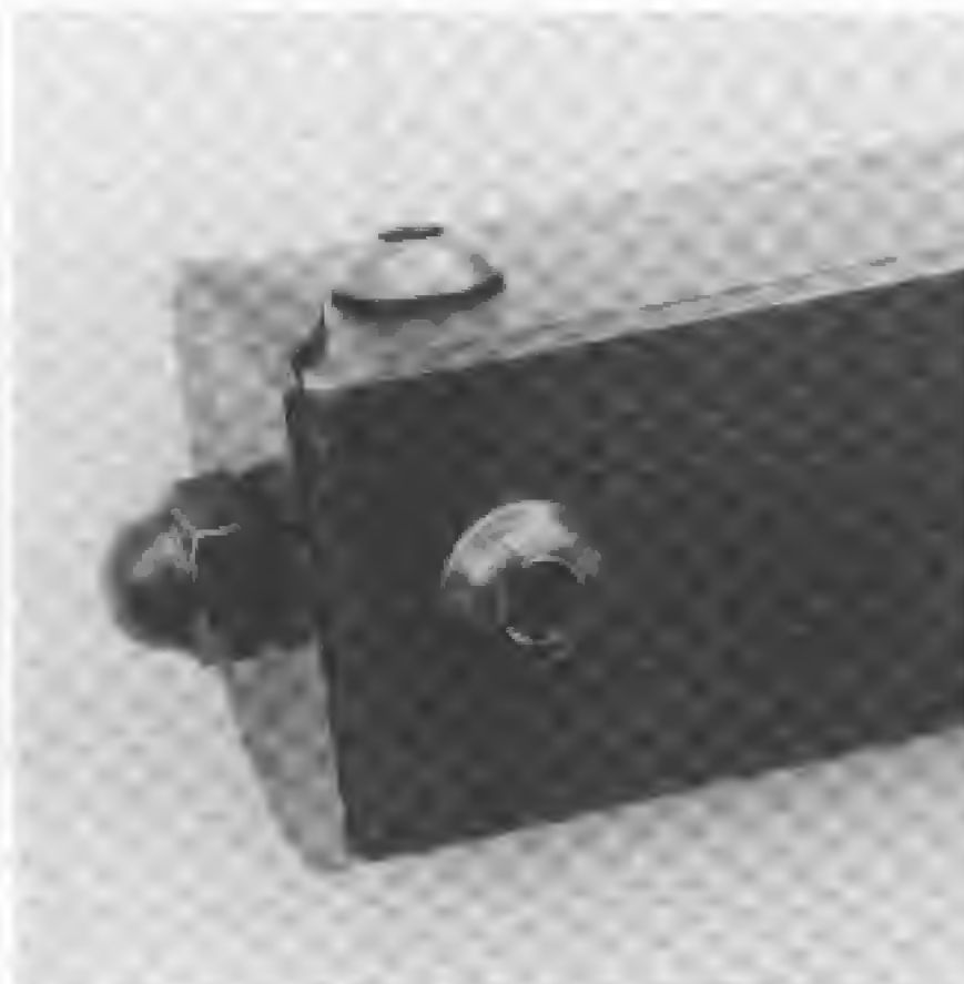
PHOTO 33: Rear view of upper receiver with modified washer (end cap) secured in place with dome nut.
