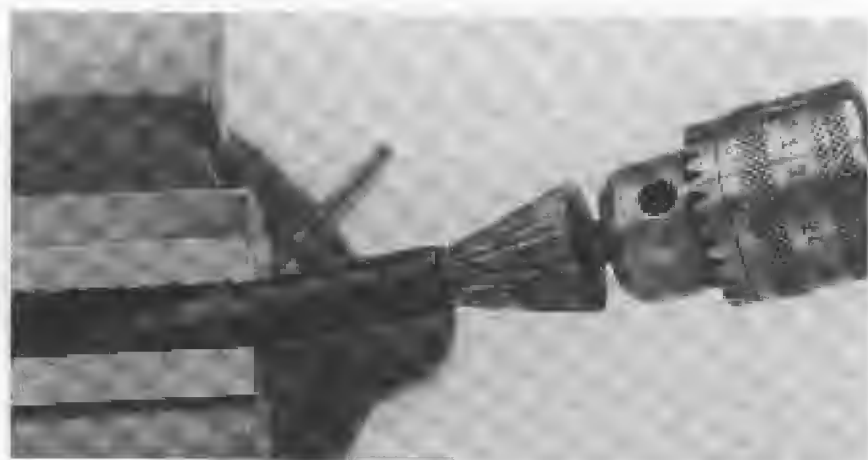
PHOTO 20: A taper is cut at both ends of the spring pin.
