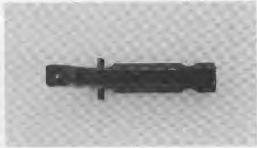
PHOTO 41: Top side view of sear. The pin should protrude the same amount on each side of the sear.
