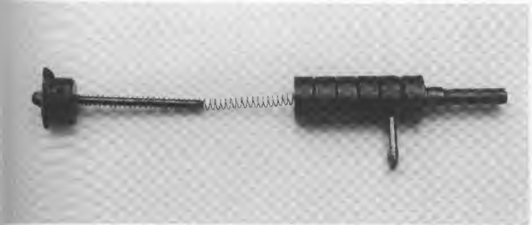
PHOTO 35: The recoil shield, guide, mainspring, and breech block shown in their respective positions.
