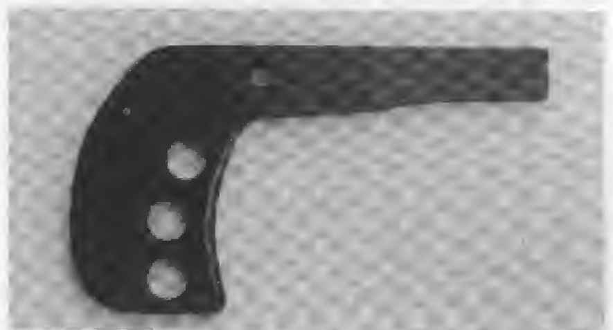
PHOTO 42: The trigger with all holes drilled.
