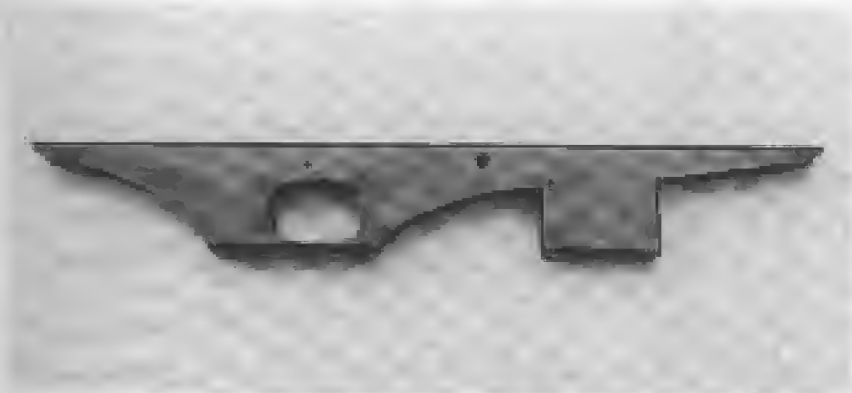
PHOTO 2: Right-side view of lower receiver after it has been filed to shape.
