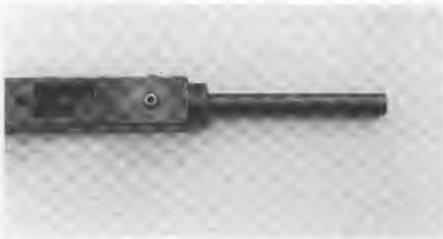
PHOTO 19: Barrel fitted to receiver.
