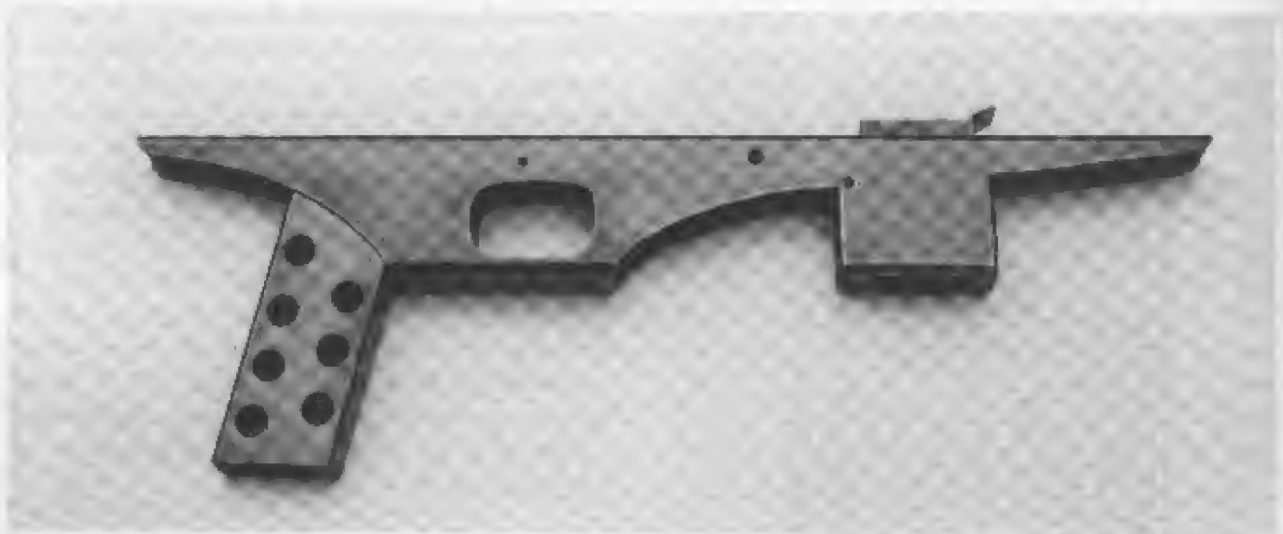
PHOTO 39: Side view of lower receiver with grip and well in position.
