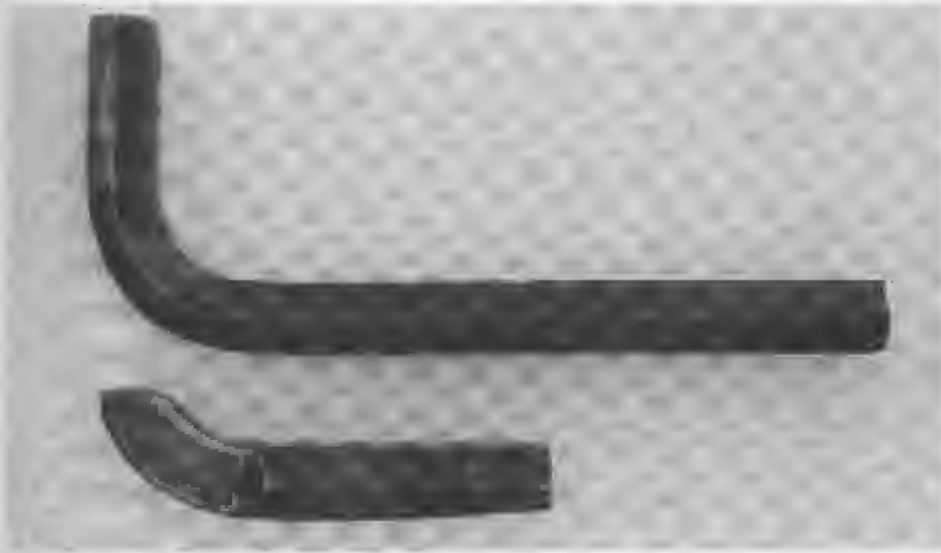
PHOTO 40: The sear before and after modification. Note the position of the spring pin.
