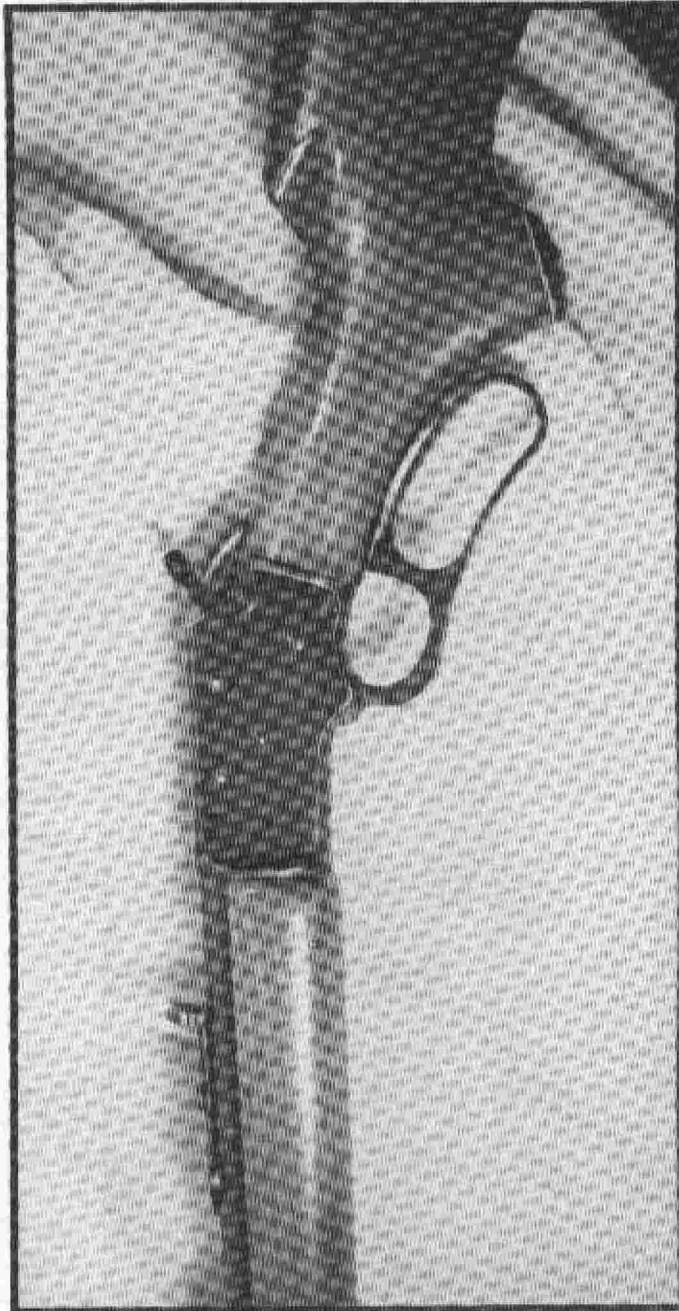
Figure 2-5 The lever action.
