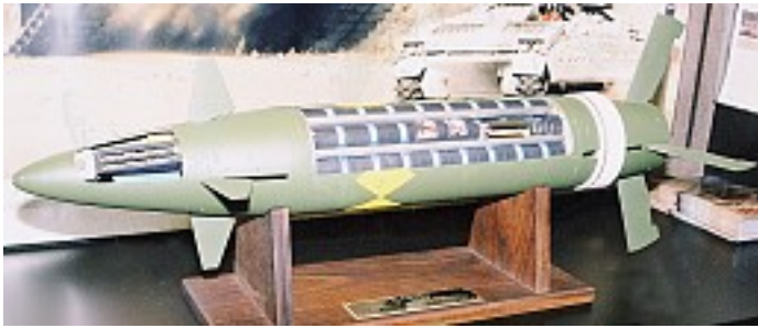
Sectioned model of a 155 mm XM982 ERDPICM projectile, showing the general layout (T J Gander) 0059314
