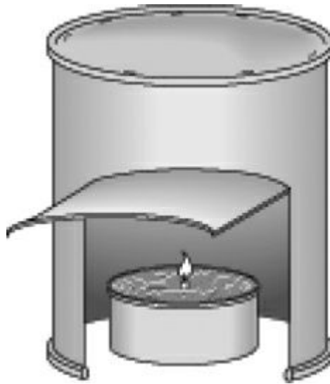
Figure 1.8 Gallon-can stove with a buddy burner.
