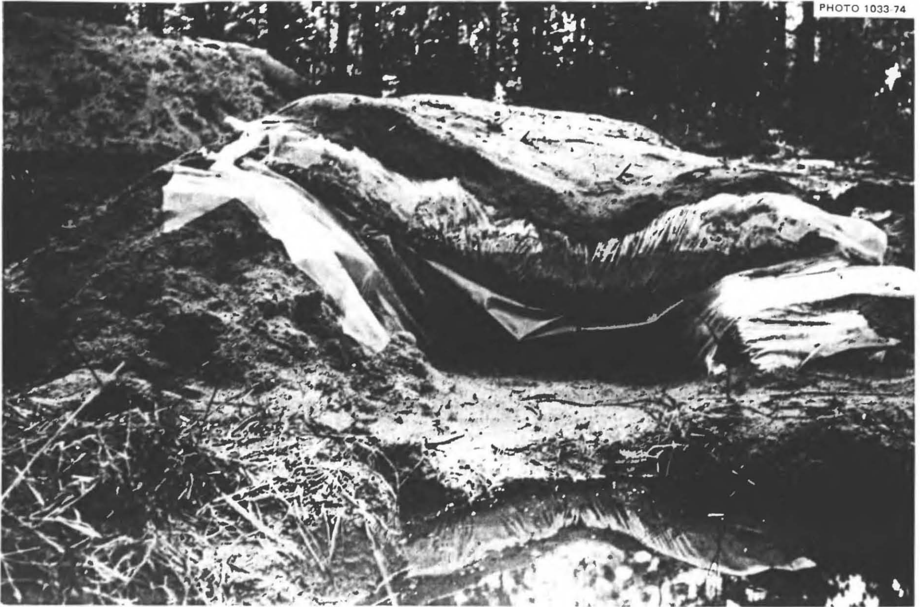
Fig. 5.61. The opposite end of the roof-door experimental setup, photographed almost one month after the beginning of this experiment. This broken-in door was unpainted. The same type of polyethylene film covered all the doors in this test. The unpainted door absorbed more moisture and was broken by the same thickness of wet earth cover that the painted doors survived. However, if the roof broke in this manner, occupants of a shelter would not have been injured, due to the fact that earth arching prevented the broken door from being dangerously depressed into the shelter.
