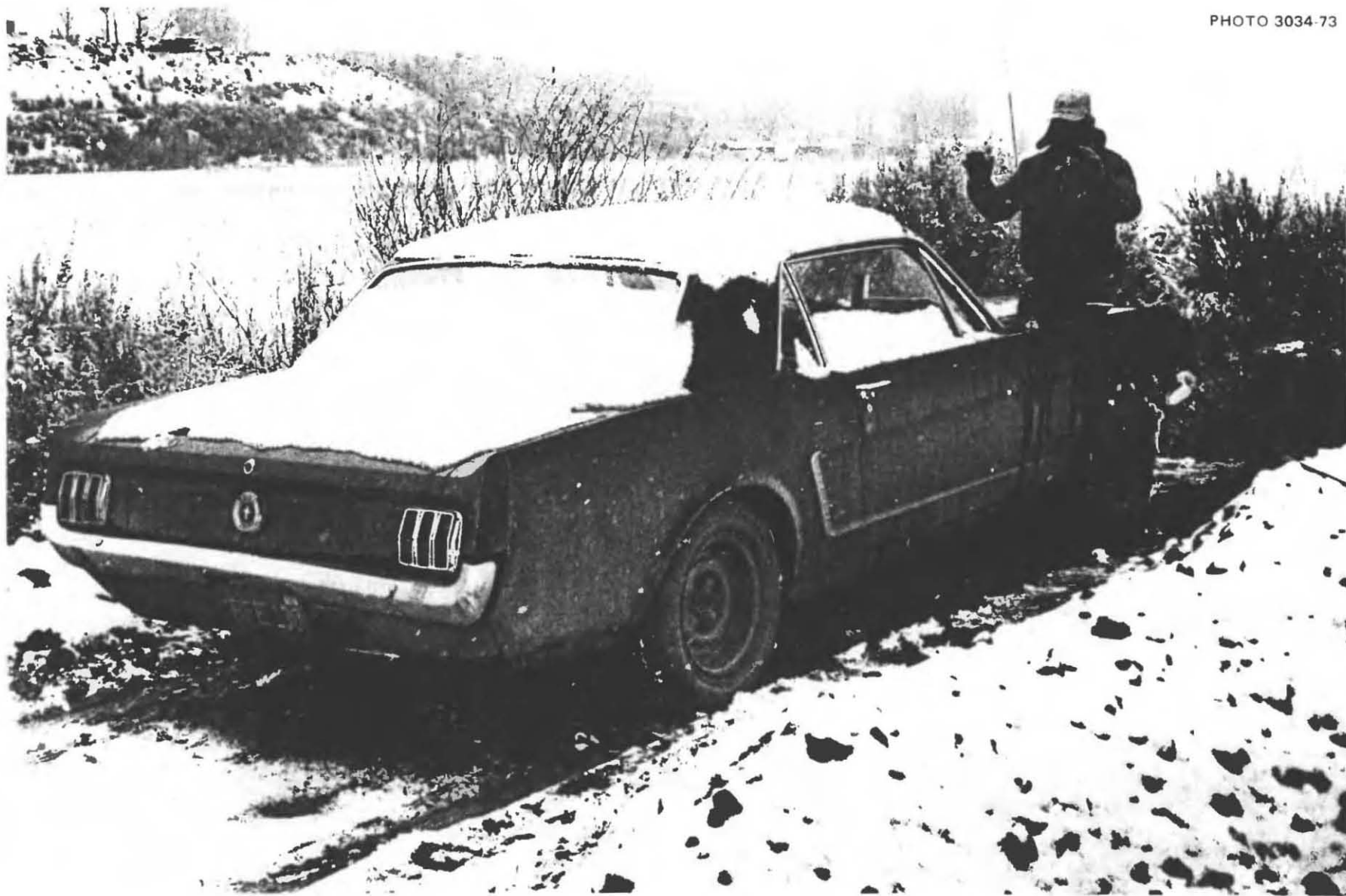
Figure 6.9. At 10:05 AM on Nov. 25, the father drove the car, on which a light snow had fallen during the previous night, evenly over the trench. Just before this, he had turned too sharply, and had come close to slipping a rear wheel into the trench – another reason for not making such trenches wider than 28 to 30 in.
