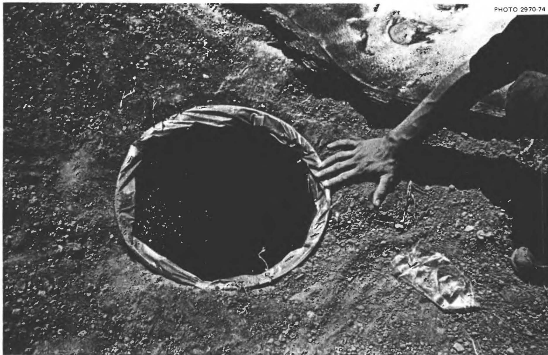
Fig. 4.36. A water storage pit lined with plastic bags, photographed 6 days after having been filled and covered. None of the approximately 25 gallons of water in this pit had leaked through the two 30-gallon trash bags (each about 1\frac{1}{4} mils thick) placed one inside the other for a pit lining.
