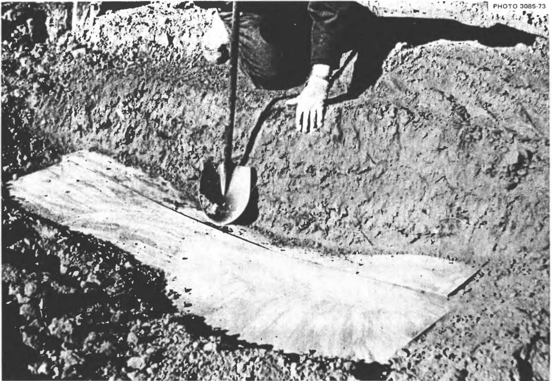
Fig. 3.7. Looking at one of the partially broken doors after the removal of earth cover 21\frac{1}{2} in. thick, measured from the man's hand to the center of the downward-bowed, unbroken upper veneer of a door. The maximum downward bowing – about 7 in. from the horizontal – occurred in the center parts of the two doors, directly under the wheels of the 8-ton backhoe.
