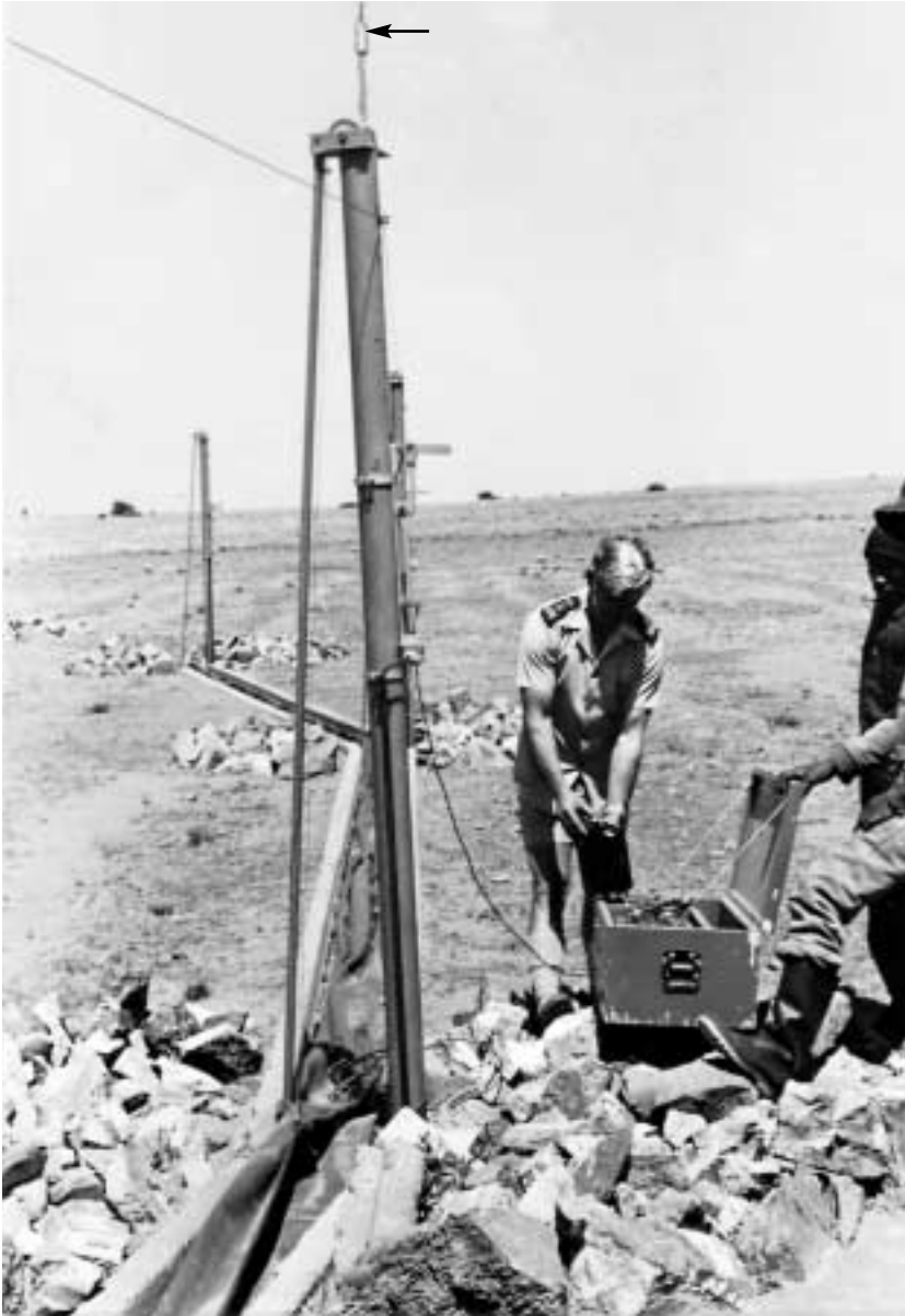
Figure 33.13 Part of a radio-controlled pop-up corral. The ditch – with the plastic sheeting, cable, metal pipe, trigger mechanism and radio antenna (see arrow) – is clearly visible.
