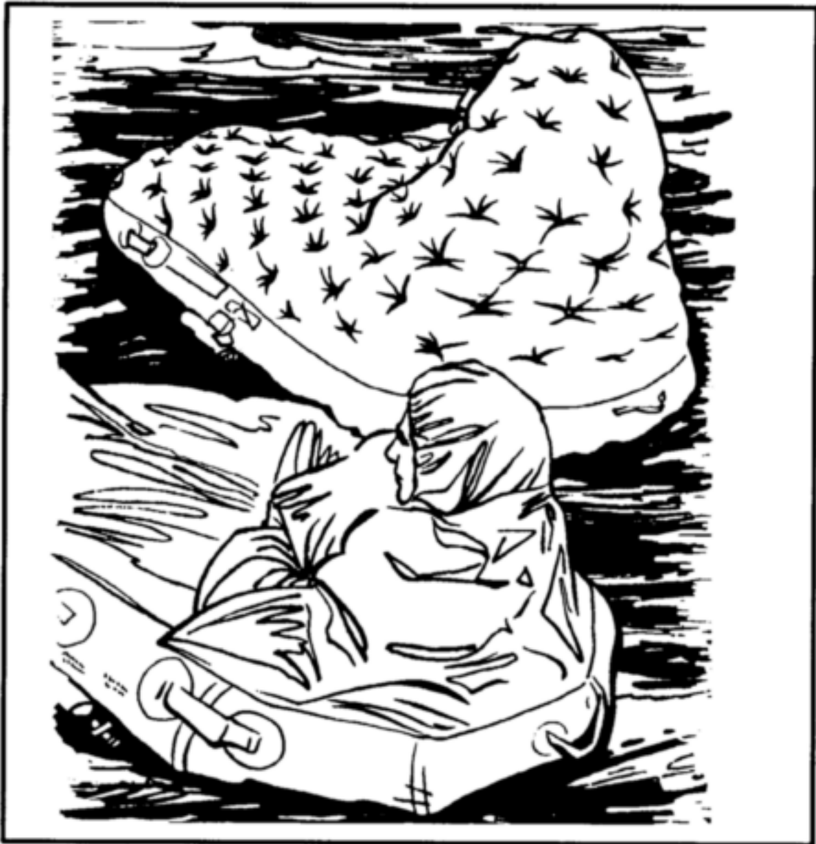
Figure 16-11. One-man raft with spray shield inflated.
